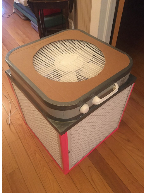
An inexpensive home-made Corsi-Rosenthal Air Filtration unit
